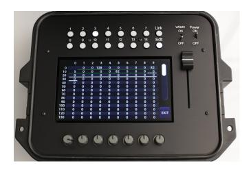
So now when I tap on address 19, you see that the red line disappears and that we get a white line starting at 19 which represents the 12channels from the skypanel in mode 1.
