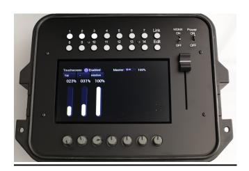
When you have selected multiple lightfixtures, You now get a shortcut to access the fixturesettings. By tapping on the nametag above the slider, you open all the options for this fixture.
