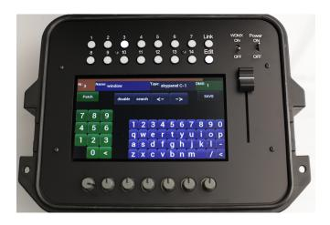
By selecting SAVE without entering a DMX Startaddress, the fixture is automatically patched to startaddres 001.
