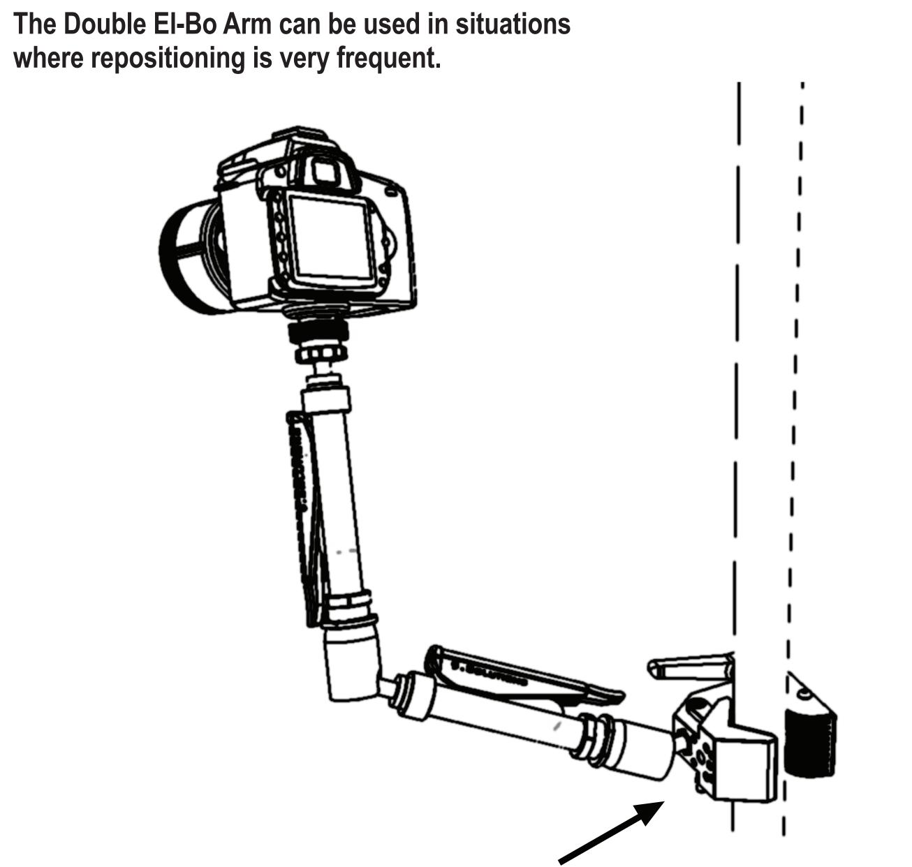
Solid mounting of the arm is best done with mounting accessories that have a 5/8" receptacle or 3/8"-16 female thread.
