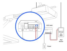
To mount on near the wall button, leave all existing wires in-place and connect one end of the red and white wires to the corresponding screws marked RED and WHITE (or R and W) on the back of the wall button, and the other end to the red and white terminals marked
