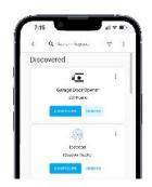
The GDO uses the built-in ESPHome integration. If it's not automatically discovered, go to Settings > Devices & Services > Add Integration > ESPHome to add it manually by IP address.
