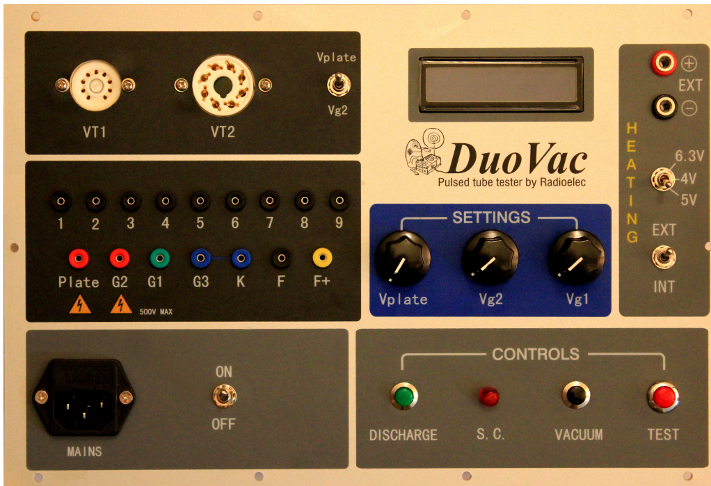
Example of a ready-to-use tube tester using this module. This item uses an interconnection matrix to adapt different types of tubes.
