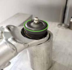
2. Press ball joint into arm until seated properly. Apply force only on the HIGHLIGHTED AREA.
