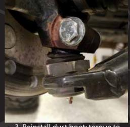
3. Reinstall dust boot; torque to 60 FT-LBS using a 1 5/8" socket.
