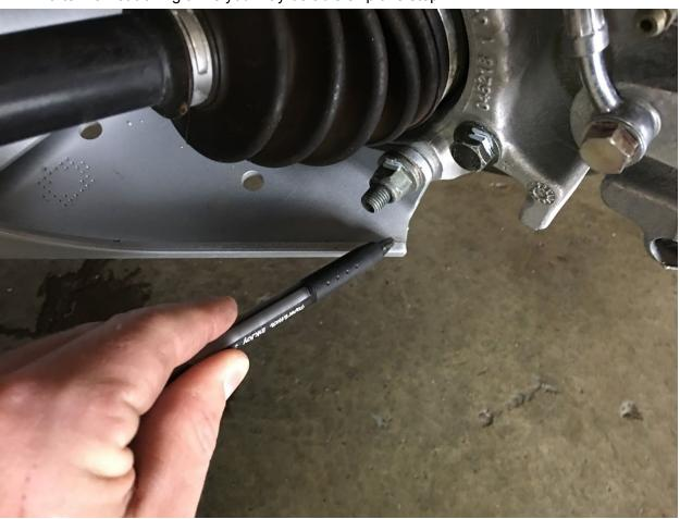
10. About 1/4" of material will need to be removed, note the edge at the tip of the pen.
