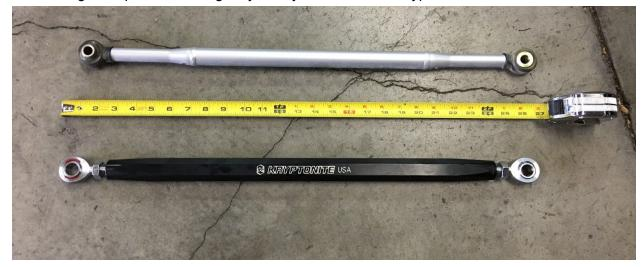
6. After you get your measurements set, finger tighten the jam nuts against the rod body for instal. The jam nuts will get tightened once the vehicle is assembled and on the ground.
