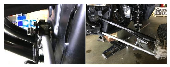
5. When each radius rod is removed lay it out on flat ground and measure the stock rods length. Duplicate the length eye to eye with the new Kryptonite rod ends.
