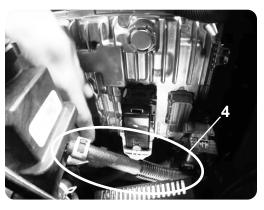
**STEP 5** - Disconnect the center, small black connector by sliding and pressing in the green tab, and then open the clamp until it disconnects.
