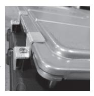
top going through the slot in the stock ECM bracket. Reinstall the 13mm bolt while making sure the Pulsar Mountaing bracket is level with the stock bracket (see picture below).
