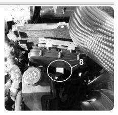
**STEP 9** - Lift Assembly up to the stock bracket, then carefully insert the ECM into the stock bracket by sliding down and back.
