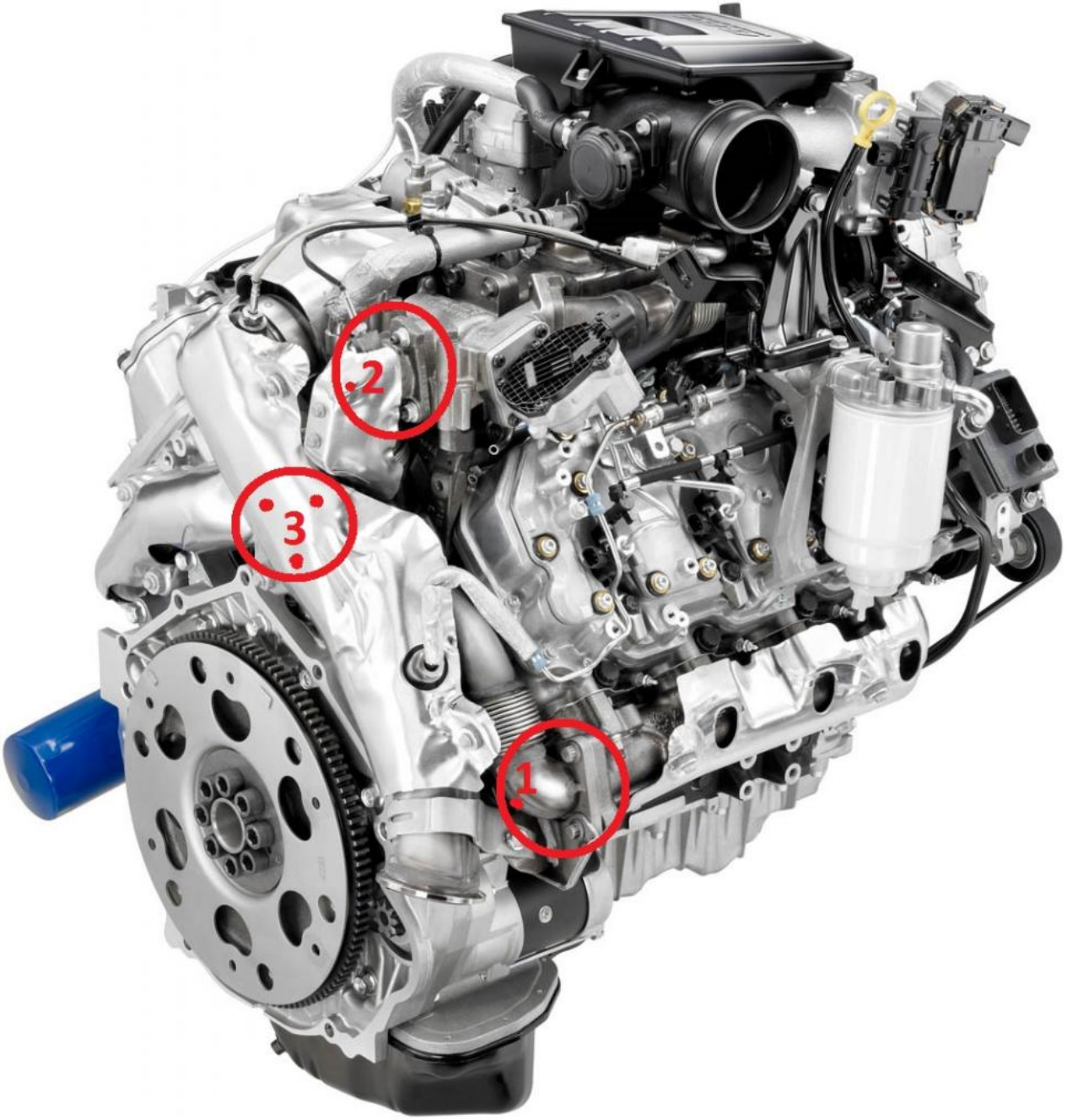
Step 14: Start by removing the 3 bolts on the intake manifold. Section 1. Keep gasket.
