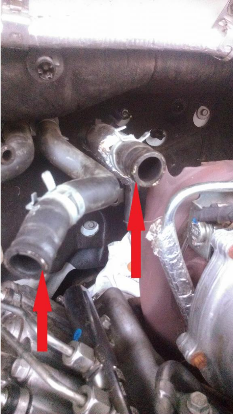
Step 19: Disconnect coolant hoses from firewall
