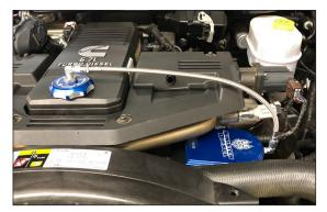
IMAGE 10 (2013-2020 Bracket Shown, installation is the same. Filter head on the 2007-2012 will be further from the engine.)
