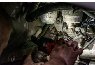
Step Sixteen: There are 8 bolts holding the factory EGR pipe to the block, remove them carefully as they have been heat cycled many times. We recommend using a torch to heat up the metal as if they break you have a lot more work.
