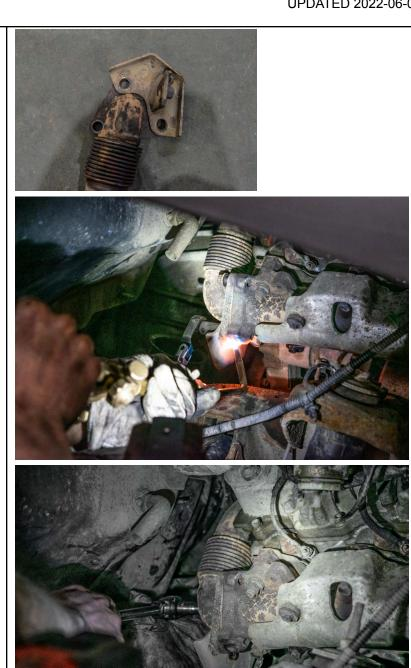
**Step Seventeen:** Now that the old pipe is out you're ready to install the new pipe. Thread in a lower bolt to hold the pipe and the gasket in place.
