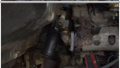
Step Nineteen: When reassembling, use the supplied coolant line to connect the two coolant hoses that were originally routed to the EGR. Most trucks require the ¾" hose, while some require 5%" hose.
