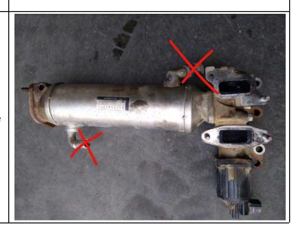
Step Ten: Remove the bolts holding the EGR to the engine, EGR cooler, and the two studs holding the EGR cooler to the up-pipe.
