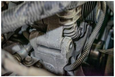
**Step Eight:** Remove the coolant lines on the front and rear of the EGR Cooler.
