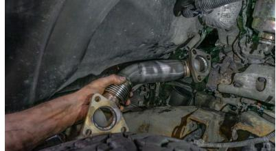
**Step Eighteen:** Now that you've got the up-pipe installed you can go for the reassembly
