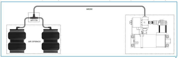
Route the airline from the compressor assembly to the air springs.
