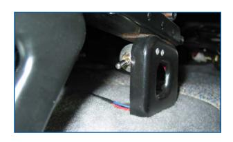
Remove the panel below the steering column. Route the wiring harness from the switch to the fuse panel.
