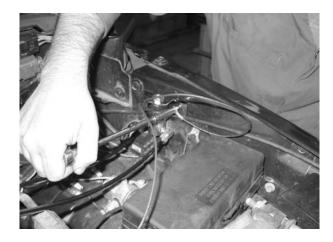
Remove the air intake plenum this will allow access to the fuel pump and intake. Remove the boost sensor line from the intake manifold and fuel pump.
