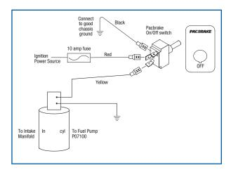
Using the 2 self tapping screws provided, mount the solenoid valve. Install one of the 2 black wires to a good vehicle chassis ground. Connect the other black solenoid wire to the yellow wire from the ON / OFF switch.
