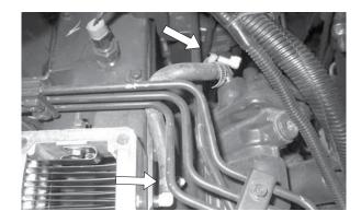
The solenoid has two 1/4" air lines, route the 29" long line (shorter of the two) connects to the fuel pump boost sensor inlet fitting. Connect the 32" long line (longer of the two) to the intake manifold boost sensor fitting. NOTE: Prior to installing the lines make sure the nut, sleeve and ferrel are in place.
