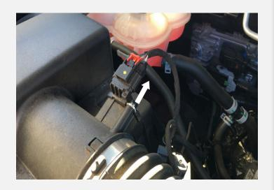
Remove the wire loom clip from the stock intake box lid.
