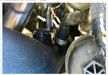
Place the Air Filter (Y) into the Airbox (A). Rotate the air filter into position as shown below and tighten the #80 Hose Clamp (Z)
