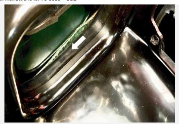
Skip to Step 25 if you installed the Box Plug (Q) in Step 20. If you installed the Auxiliary Scoop (P) use install the 1/4-20 Screws (M), Lock Washers (N), and Washers (O) with an 11mm Socket/Wrench from inside the Airbox (A).
