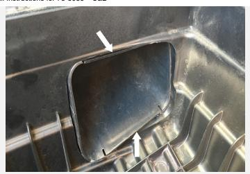
Remove the stock intake box from the vehicle, then remove the stock air inlet from the fender wall. Be careful not to pull too hard when removing the stock intake box. Remove a section of the intercooler piping for more clearance if necessary.
