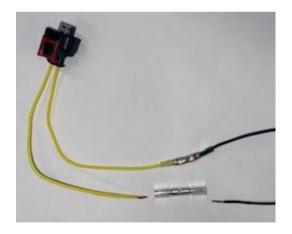
2. Connect new pigtail to injector
