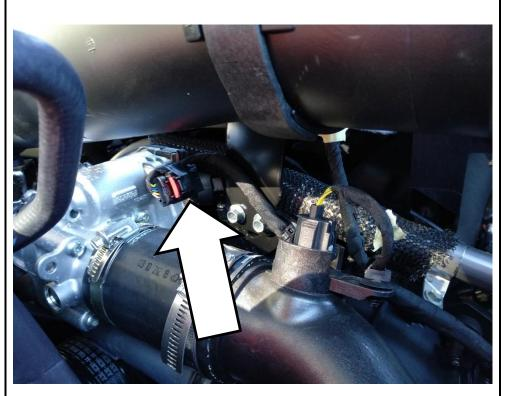
2. Locate engine crankshaft position sensor on the motor. Connect the supplied BD PAS wiring harness inline so that the BD harness connects to the crankshaft position sensor and to the vehicles original wiring.
