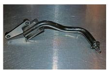
Using a 1/2" drive ratchet or breaker bar, release the serpentine belt tensioner and slide the belt off of one of the accessories before releasing the tensioner. Remove the tensioner mounting bolt. Remove the tensioner and serpentine belt from the vehicle.
