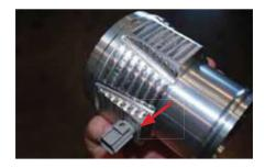
With a pick or other small-ended tool, carefully remove the O-Ring from the inside of the factory intercooler pipe. Clean the O-Ring of any oil or debris and apply a small amount of Vaseline or Assembly Lube/Grease to the O-Ring. Install the O-Ring to the groove inside the HSM throttle adapter by starting on one side and working all the way around, ensuring it is fully seated in the groove.
