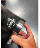
Note: Make sure when installing the clamp on the intercooler end of all boots to be sure the clamp is pushed up close against the intercooler outlet as shown, so the intercooler outlet does not cut the boot if the clamp is tightened too far out.
