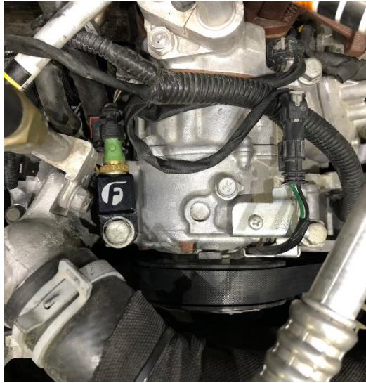
Fig. 17: Fuel temperature sensor block location
