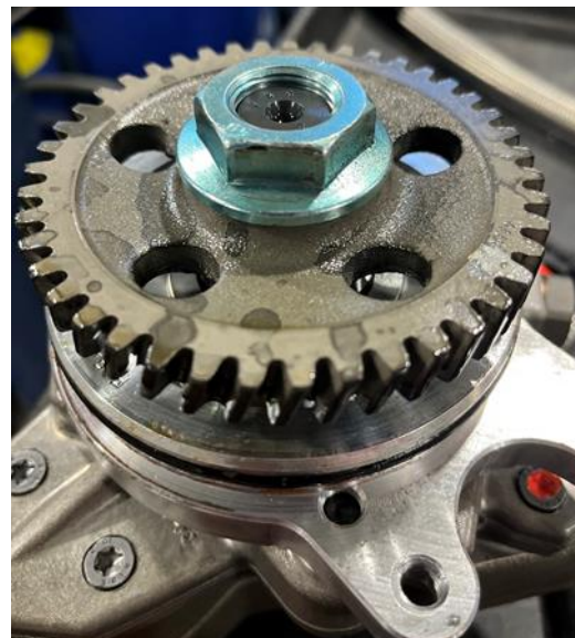
Fig. 12: Install the CP4 nut onto the CP3
