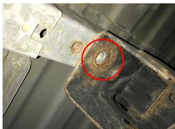
STEP 4: Disconnect the fuel filler neck from the bed.
