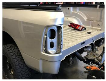
STEP 3: Remove the bolts that retain the bed of the truck to the frame. For the short bed model, there will be 6 fasteners. For the long bed model, there will be 8 fasteners.
