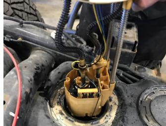
STEP 10: Clean the tank sealing surface and place your <u>new</u> o-ring supplied in the kit for the PowerFlo lift pump onto the top of the tank.
