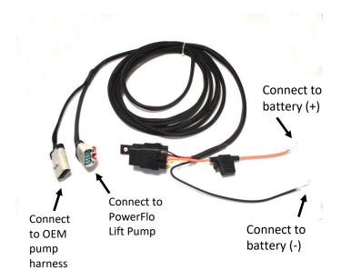
STEP 12: Neatly route the wiring harness from the driver side battery compartment to the OEM pump connection. Route the harness in a manner that it will not interfere with any moving parts and retain it with zip ties along the main electrical harness of the truck routed to the rear of the truck.
