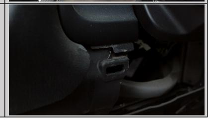
Step Five: Trim the plastic on the kick plate using an exacto knife to make room for the switch (pictured is before and after)
