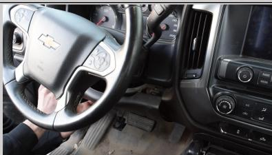
**Step Four:** Trim the plastic on the right side of the driver side receptacle for the kick plate clip.
