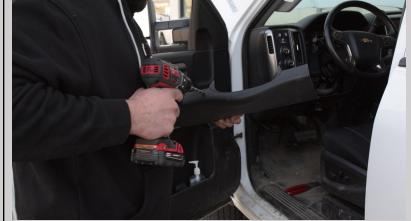
Step six: Drill the hole using a % bit through the front of the kick panel to line up with the plastic you just trimmed
