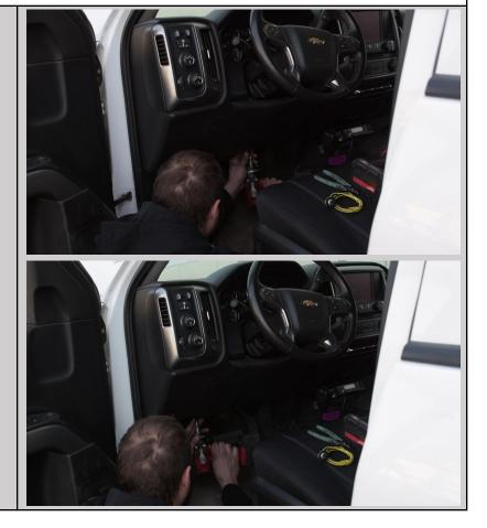
**Step Two:** Remove your Hood latch. There should be two small clips holding it in place.
