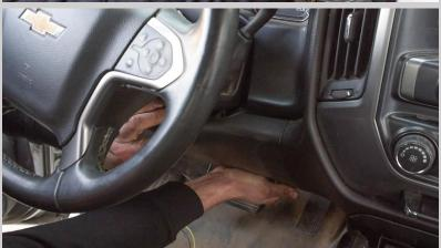
**Step Nine:** Locate a grommet on the firewall and make a hole for the wires to go through (we used a blank)
