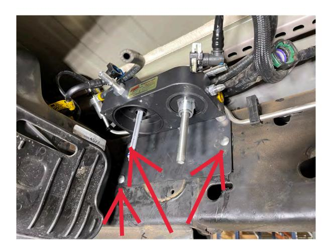
NOTE: REMOVING THE LOWER FILTER HOUSING FROM THE FASS ASSEMBLY CAN HELP OPEN ADDITIONAL SPACE FOR INSTALLING THE FASS ASSEMBLY THOUGH IT IS NOT NECCESARY.
