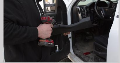
Step six: Drill the hole using a % bit through the front of the kick panel to line up with the plastic you just trimmed
