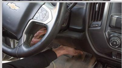
**Step Nine:** Locate a grommet on the firewall and make a hole for the wires to go through (we used a blank)
