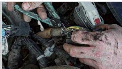
**Step Fifteen:** Count 11 wires up in the row closer to the front of the truck to find your pin
