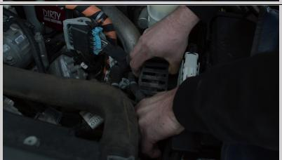
Step Twelve: By releasing the red lock on the back of the harness clip, remove the middle connector on the PCM
