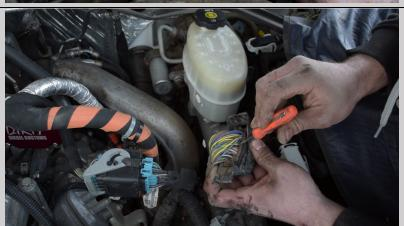
**Step Sixteen:** In order to run the wire through the hole you will have to drill out the plastic plug that blocks it
