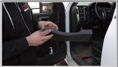
Step Eight: Plug the wires into your switch, run them ahead of the panel and reinstall the kick plate with screws and hood release lever
