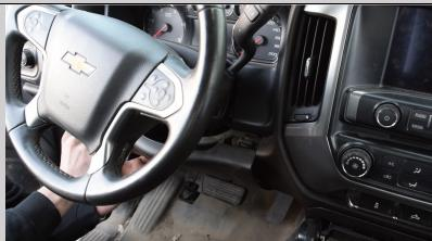
**Step Four:** Trim the plastic on the right side of the driver side receptacle for the kick plate clip.
