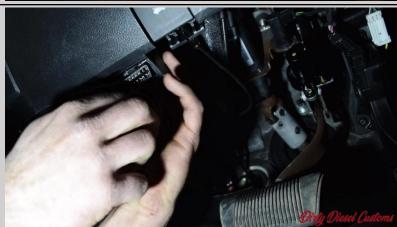
**Step Fourteen:** Plug the factory OBD2 into the receptacle on the AutoCal wiring
