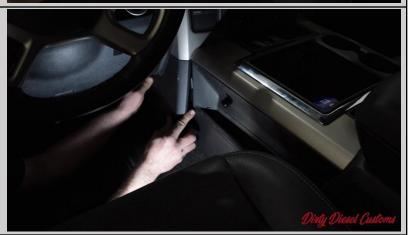
**Step Twelve:** Replace the factory OBD2 port with the AutoCal port by depressing the two clips on the side and sliding out the factory port
