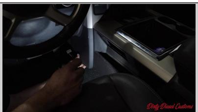
**Step Ten:** Run the wiring for the switch through the kick plate up to the opening of the panel where the switch is going
