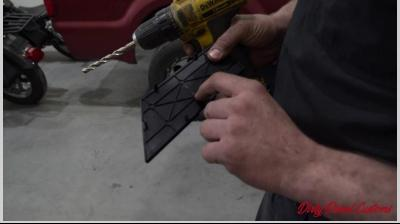
**Step Three:** Drill the 3/8<sup>th</sup> hole for the switch from the back of the panel
