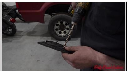
**Step Four:** Trim the 1/8<sup>th</sup> inch tab off the switch as the locking washer and nut are adequate to hold the switch in place
