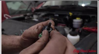
Step Seven: Place the switch through the back of the panel and use the lock washer and nut on the front to secure it together. Once it is snug by hand, do a ½-3/4 turn on the nut to tighten. Be careful of the plastic screws to not strip the unit
