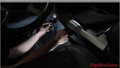
**Step Eleven:** Plug the wiring of the switch into the switch and reinstall both plates
