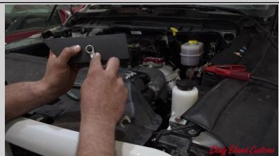
**Step Eight:** Using the supplied Allen key, secure the knob to the switch and confirm the correct switch count
