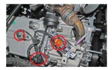
Step 14: Unplug the PCM harness from the PCM and secure out of the way.
