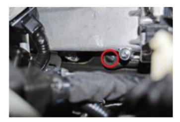
Step 17: Remove the seven bolts that hold the egr cooler in place using an 8mm socket.
