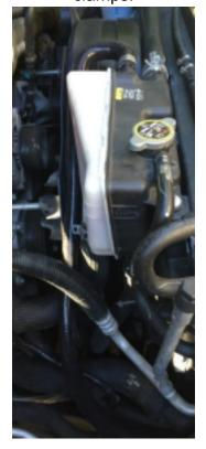
**Step 10**: Disconnect the quick connect coolant line from the metal stand pipe that is between the egr cooler and the intake manifold.
