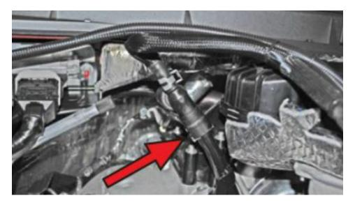
Step 25: Reconnect the pcm harness. Make sure the plugs are fully seated.
