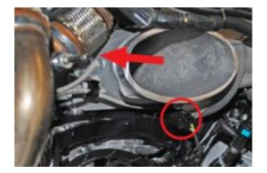
**Step 12:** Remove the longer egr pipe that is fastened with 5 6 mm bolts using an 8mm socket.
