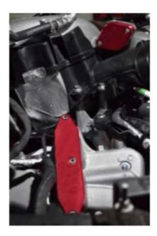
**Step 24:** Reconnect the quick connect coolant hose to the metal standpipe. Reconnect the top line to the brass barbed fitted from step 8.
