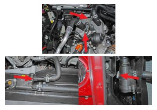
**Step 8:** Remove the three hose clamps on the 5/16" coolant hose and remove the tee. Install the supplied 5/16" straight barbed fitting and two small stainless steel hose clamps. Note on 2015-2016 trucks, use the supplied 3/8" straight hose barb and two small stainless steel hose clamps to connect the two radiator overflow hoses.
