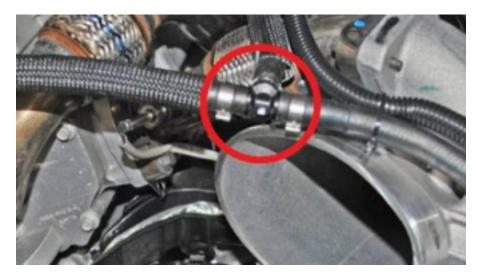
**Step 9:** Install the supplied <sup>3</sup>/<sub>4</sub>" molded silicone hose from the degas tank to the disconnected port near the bottom of the radiator that was removed in Step 7 using the supplied hose clamps.
