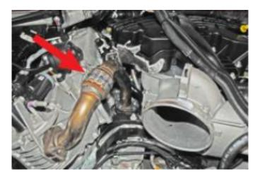
**Step 13**: Unplug the harnesses on top of the egr cooler and vacuum hose by first removing the 90 degree fitting. Install the supplied vacuum hose cap and zip tie the harnesses to the pcm harness.
