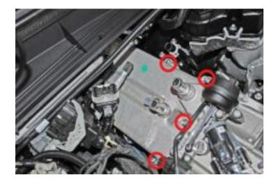
**Step 18:** Remove the 10mm nut that retains the EBP hard line to the back of the EGR cooler. Note that on 2015-2016 trucks, the nut is a 12mm.
