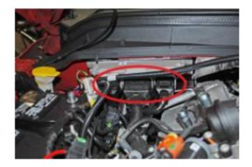
Step 15: Remove the two bolts that secures the wiring harness to the egr cooler using an 8mm socket.
