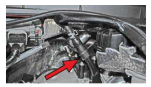
**Step 11:** Disconnect the egr temperature sensor using a 14mm wrench and remove the short egr pipe using an 8mm socket.
