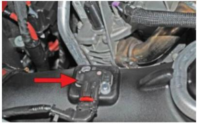
Step 4: Remove the two bolts that hold the air intake resonator and air filter box using an 8mm socket.
