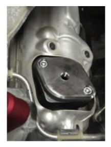
**Step 22:** Install the supplied egr cooler pass through plate using three of the M6x30mm bolts with a 5mm allen wrench.
