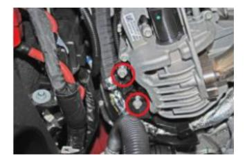
**Step 16:** Remove the two clips on the heat shield that are located on the passenger side under the egr cooler.
