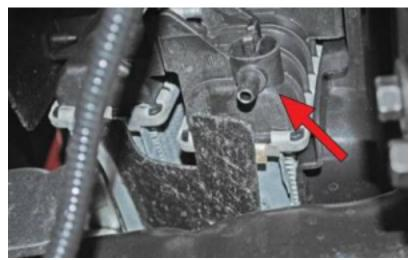
Step 3: Unplug the MAF sensor that is located on the intake by releasing the red locking tab.
