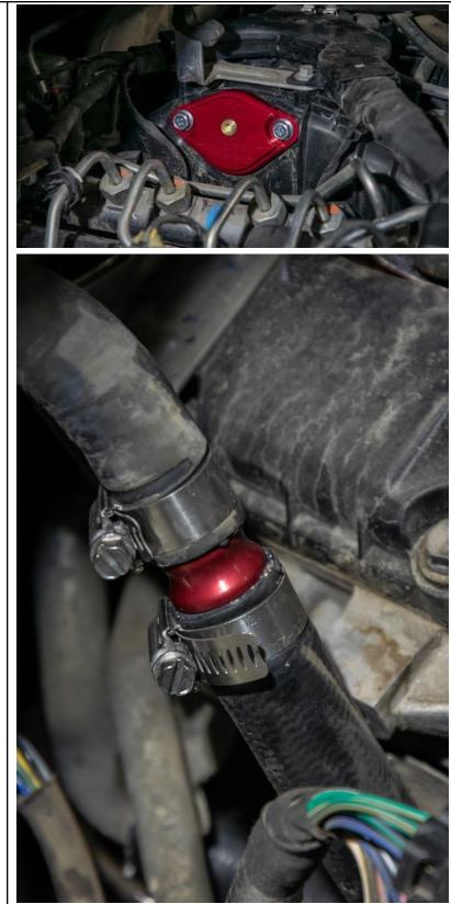
**Step Fourteen:** Install the blocker plate on the intake manifold.
