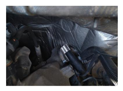
**Step 8:** Route the 5/8" hose down to the frame rail and secure it at the top using the supplied hose clamp, and along the length using zip ties.
