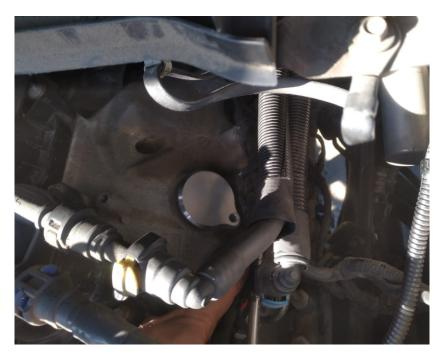
**Step 7:** Install the Flow Through Plate using the supplied SHCS and a 5mm allen driver. At this point you can either install it with the hose bung pointing to the fore or aft of the vehicle, depending on how you want to run the drain hose. Either configuration works, so it's up to you!
