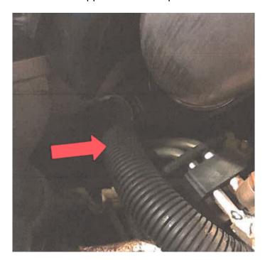
**Step 4:** Remove the 4 bolts that fasten the ccv housing to the valve cover using a 10 mm socket. Remove the ccv housing by pulling up, then towards the front of the vehicle. Use caution as excess oil from the ccv separator will drain out.
