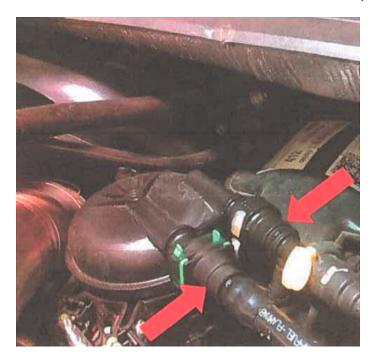
**Step 2:** Using an 11mm socket, loosen the factory hotside intercooler pipe clamp from the intercooler and rotate it out of the way.
