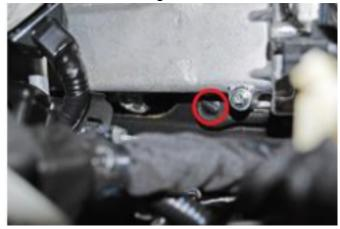
**Step 12:** Remove the seven bolts that hold the egr cooler in place using an 8mm socket.
