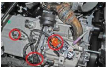
Step 9: Unplug the PCM harness from the PCM and secure out of the way.
