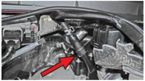
**Step 19:** Connect the coolant hose on top of the quick connect to the coolant Tee previously mentioned in step 4. You can remove the push in zip tie and tidy the coolant hose routing with provided zip ties. These hoses should be routed roughly as shown below.
