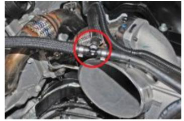
**Step 5:** Disconnect the quick connect coolant line from the metal stand pipe that is between the egr cooler and the intake manifold.
