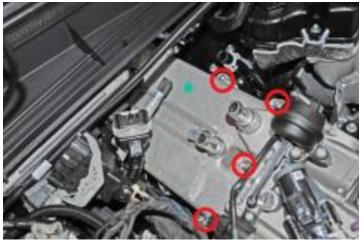
**Step 13:** Remove the 10mm nut that retains the EBP hard line to the back of the EGR cooler. Note that on 2015-2016 trucks, the nut is a 12mm.
