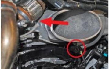
Step 7: Remove the longer egr pipe that is fastened with (5) 6 mm bolts using an 8mm socket.
