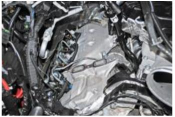
**Step 15:** Install the supplied exhaust manifold block off plate and factory gasket using two of the supplied M8x25mm flange head bolts with a 12mm socket. If not installing an aftermarket 1/8" EGT Probe, install the supplied EGT Probe Adapter with a 5/8" socket and one of the factory EGT sensors from the DPF system.
