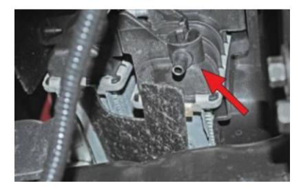
**Step 3:** Loosen the two clamps on the air intake tube using a 7mm socket and unplug the MAF sensor that is located on the intake tube by releasing the red locking tab. Remove the air intake tube.
