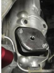
**Step 16:** Install the supplied egr cooler pass through plate using three of the M6x30mm bolts with a 5mm allen wrench.
