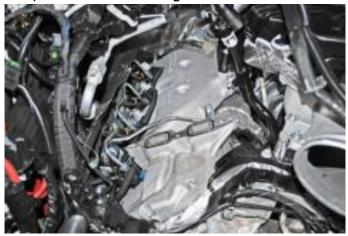
Step 15: Install the supplied exhaust manifold block off plate and factory gasket using two of the supplied M6x20mm bolts with a 5mm allen wrench. If not installing an aftermarket 1/8" EGT Probe, install the supplied EGT Probe Adapter with a 5/8" socket and one of the factory EGT sensors from the DPF system.
