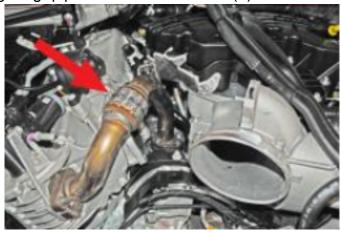
Step 8: Unplug the harnesses on top of the egr cooler and vacuum hose by first removing the 90 degree fitting. Install the supplied vacuum hose cap and zip tie the harnesses to the PCM harness.
