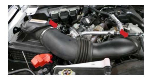
Step 4: Remove the three hose clamps on the 5/16" coolant hose and remove the tee. Install the supplied 3/8" straight barbed fitting and two small stainless steel hose clamps.
