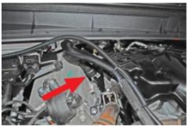
Step 6: Disconnect the egr temperature sensor using a 14mm wrench and remove the short egr pipe using an 8mm socket.
