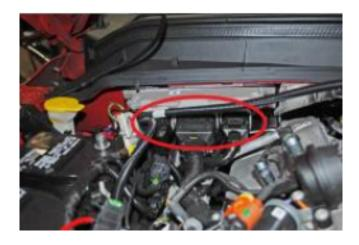
Step 10: Remove the two bolts that secures the wiring harness to the egr cooler using an 8mm socket.
