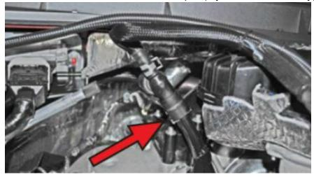
Step 19: Reconnect the PCM harness. Make sure the plugs are fully seated.
