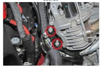
Step 11: Remove the two clips on the heat shield that are located on the passenger side under the egr cooler.
