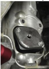
Step 16: Install the supplied egr cooler pass through plate using three of the M6x30mm bolts with a 5mm allen wrench.
