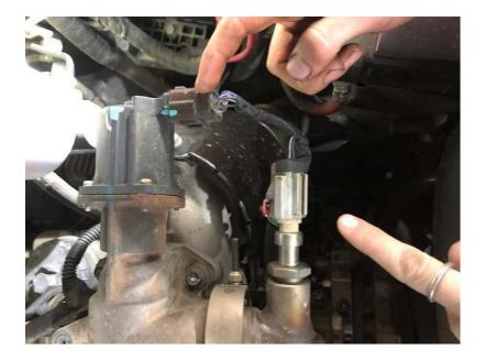
**Step 4:** Once the EGR is disconnected, remove (x4) bolts holding the EGR Valve on top of the
