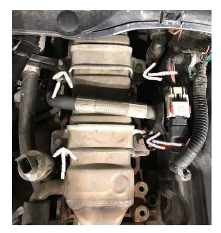
**Step 26:** Unbolt the four (x4) 10mm bolts that hold down the EGR Cooler.
