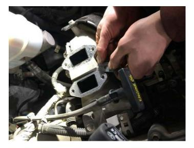
Step 9: Once the surface is as clean as possible, place both new gaskets on with the larger
