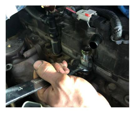
**Step 36:** Grab the Coolant Nipple you removed in the last step and remove the O-Ring and put Teflon Tape on the threads and have it ready to place into the plug you are removing in the next step.
