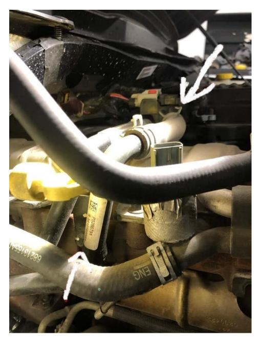
Step 15: Remove the intake tube and smaller crankcase tube from the air filter to the turbocharger.
