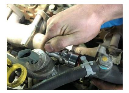
Step 39: Get out your Black Steel Bracket and attach it to the block with some M8 Socket head cap screws. These threaded holes in your block can be a bit cruddy, so wash it out, blow it out, use a tap and chase it out, whatever, just make sure you're not ruining the threads. When installing, make sure the hose adapter goes into its slot. Just drop the bracket down onto the installed hose adapter.
