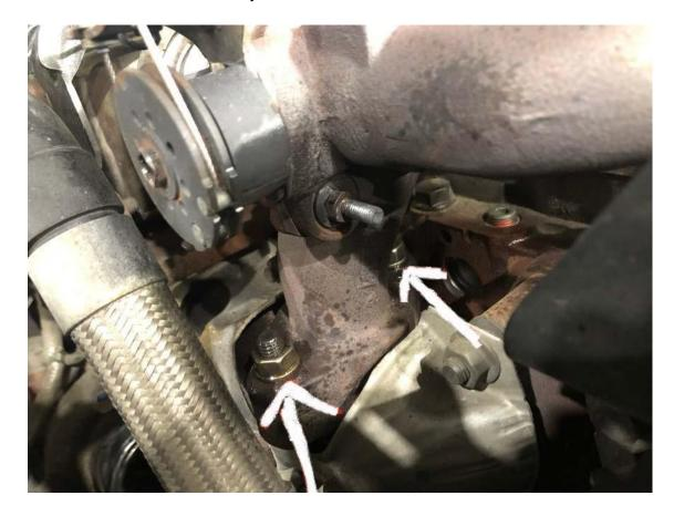
Step 21: Break the accessible 15mm nut free, then, you'll then need a stubby 15mm wrench to get the remaining nut. We like to use a pry bar on the wrench to break it free, just set the wrench on the nut and get the pry bar in from the top and crack it. Just make sure you're not prying on anything that can break!
