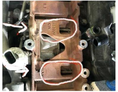
**Step 33:** Now you're ready to install the second larger Steel Plate. If you have a pyrometer, you can install the bung on the plate and install your pyro. If not, just make sure you install the <sup>1</sup>/<sub>8</sub>" NPT plug snug in place and **Torgue the plate to 37ft-lbs.**
