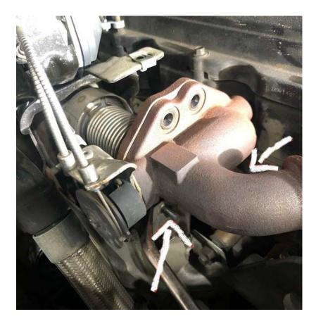
Step 18: Now you can pry the heatshield off the one stud and bend it out of the way to
