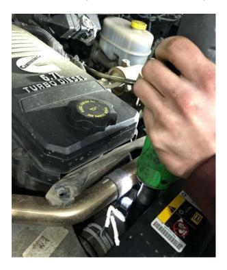
Step 6: Now, on the far left side of the EGR crossover tube undo the v-band clamp using an
