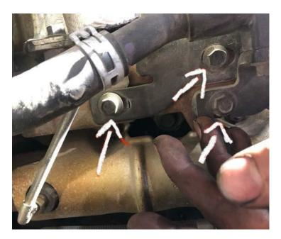
Step 24: Pull off the Bypass Valve Assembly including the front section of the cooler
