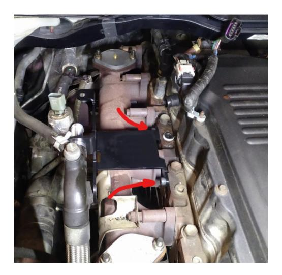
**Step 40:** Now, you can bolt up the transmission dipstick to the top of the bracket using a <sup>1</sup>/<sub>4</sub>" bolt and nut.
