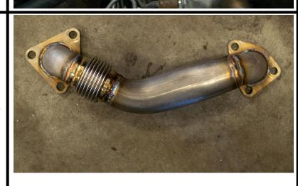
**Step Twenty:** Now install the new up pipe that goes directly to the turbo.
