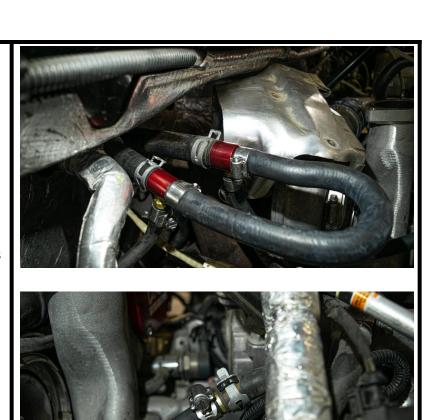
Step Nineteen: Next, install the coolant re-route kit on the hoses coming out of the firewall.
