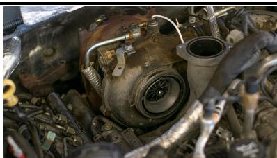
**Step Eighteen:** On the intake, behind the A/C compressor, install the blocker plate.
