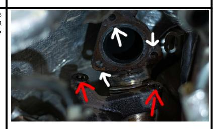
Step Fourteen: Once you have the up-pipe bolts off, you will need to separate the two halves of the EGR cooler. There are four bolts connecting them with 13mm heads. The bottom two are only accessible once the whole setup is disconnected from the motor, which is why this is the final step.
