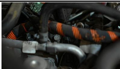
**Step Ten:** Unhook the coolant lines to the EGR cooler
