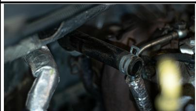
Step Sixteen: Now you're moving on to the downpipe. First off you'll have to head over to the driver's side firewall and undo this electrical module. It's easier to take this off than the sensor on the downpipe, take them off together.
