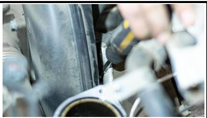
**Step Nine:** Un-bolt the bracket holding the dipstick on the passenger side
