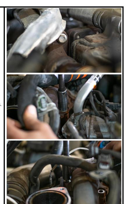
Step Eleven: Remove the EGR bypass pipe held on by five bolts. It runs from the passenger side by the up-pipe to the driver's side near the A/C compressor.
