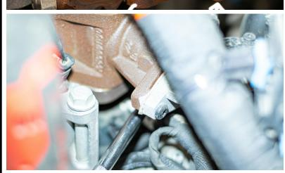
Step Thirteen: The hardest bolts to get are the up-pipe to the EGR cooler. The first image shows the setup already disconnected so you can easily reference the locations. There are 3 bolts (white arrows) connecting the cooler to the up-pipe and then two bolts (red arrows) connecting the cooler to the bracket. The rear 3 usually requires a combination of a wrench and pry bar to remove. (shown to the right) Be careful and take your time! They are prone to breaking.
