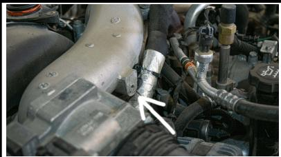
Step Four: Remove these connectors from the top of the motor. Disconnect the throttle valve near the passenger side, and the green connector back towards the firewall.
