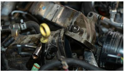
Step Fifteen: In order to take off the downpipe you will need to remove the hard coolant pipe that runs down the back of the block. It's held by a single 13mm bolt. Be careful as the O-Ring can get damaged, if damage occurs you will have to replace it.
