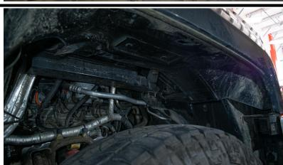
**Step Three:** Remove the top cover and intake hose of the motor. Then un-bolt the wiring harness from the intake pipe.
