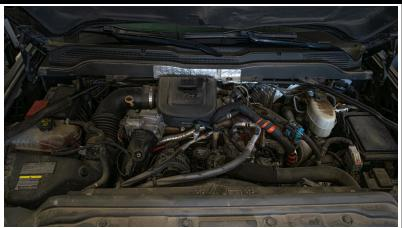
Step Two: Remove the fender liner with its T15 Torx bolts and hit every single bolt of the turbo/downpipe with penetrating fluid. The longer the penetrating fluid can sit on the bolts the less likely they are to break on you. Breaking bolts during this job is common.
