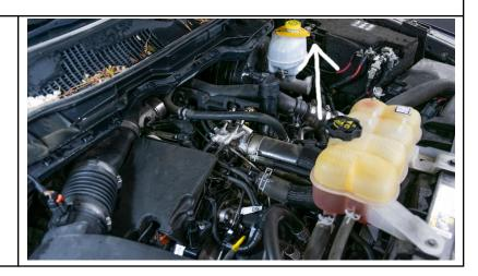
Step Two: Remove the Top engine cover by pulling up on it.
