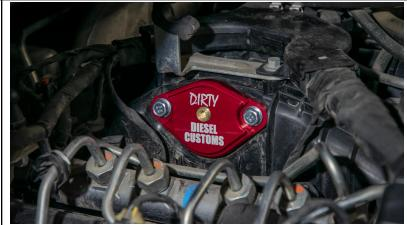
**Step Fourteen:** Install the blocker plate on the intake manifold.
