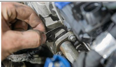
**Step Six:** Remove the crossover pipe to the intake
