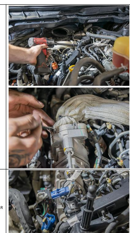
**Step Seven:** Disconnect the electrical connections to the EGR
