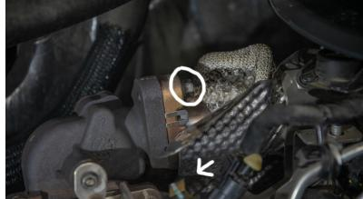
Step Ten: Remove the bolts holding the up pipe to the EGR Cooler. There are two bolts and then a T40 torx bit holding it on the bottom. Shown in the 3rd picture are the bolt locations.
