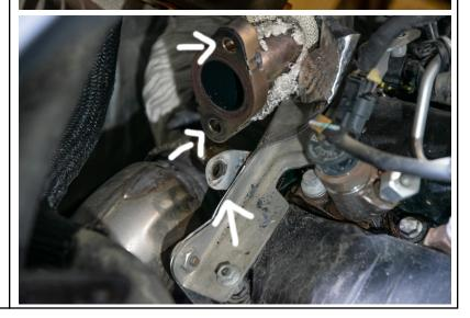
**Step Eleven:** Remove the 3 13mm bolts that hold the EGR cooler to the head
