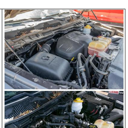
**Step Three:** Remove the intake piping from the air box to the intake manifold.
