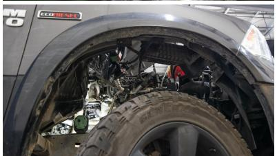
Step Thirteen: Remove the 3 bolts that hold the EGR pipe to the manifold. We highly recommend heating them with a torch + penetrate spray. Then install the blocker plate in its place, reusing the factory gasket.
