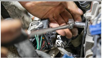
Step nine: Remove the two torx bits that hold on the vacuum diaphragm at the rear side of the EGR cooler.
