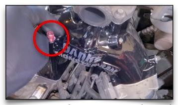
**103. Put Long Bolt Into Front Corner by Hand** This will help hold the Monster-Ram in place. Then do the same for the long bolt on the backside. Followed by the two smaller bolts.
