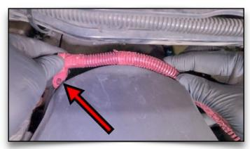
**98. Push Cable Ties Onto Studs**Use the supplied extension to reconnect the EGR pipe and tube sensor.
