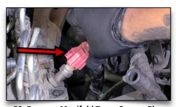
53. Remove Manifold Temp Sensor Plug
