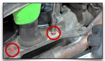
**10. Remove Bolts Holding Crossover Bracket** This bracket will not be reused.
