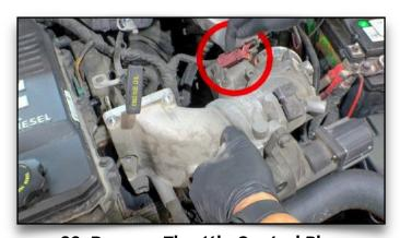
**39. Remove Throttle Control Plug**Now that the elbow has been leaned forward, you can easily reach this plug.
