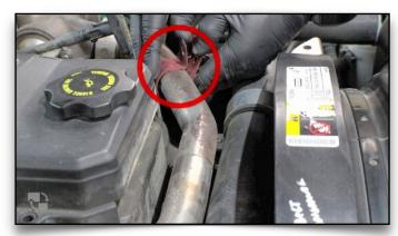
14. Remove and Dispose EGR Tube P-Clamp
