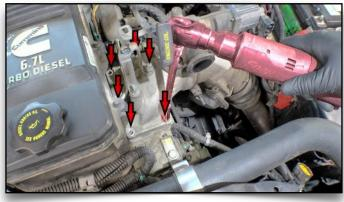
37. Remove 6 Bolts on Elbow
