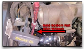
115. Tighten 12V Heater Nut
