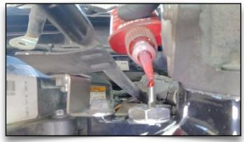
114. Apply Red Thread Locker to Coil Heater
