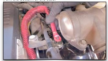
Bend 12V Cable around as shown over the stud.
