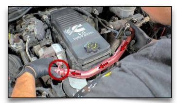
**25. Release Passenger Side EGR Clamp**Apply pressure to keep the gasket in place and Keep your hand under the passenger side clamp to prevent the flat EGR gasket from falling into the engine bay.
