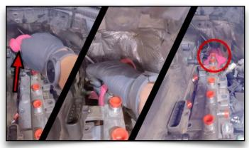
**61a. Place Rag At Rear of Fuel Rail**There will still be fuel in the rail, and it'll leak out in the next step if you don't do this.
