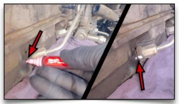
55. Paint Marker Line Across Threaded Insert & Cylinder head
