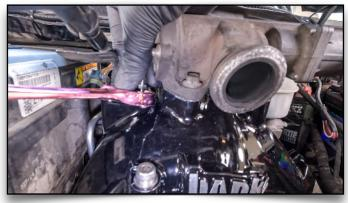
106. Tighten Coil Heater By Hand
