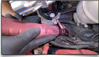
112. Tighten Boost Tubes Clamp
