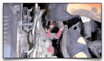
**50. Remove Cable Ties from Driver Side Studs**
