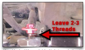
12V cable should be sandwiched in-between both nuts, away from metal contract.
