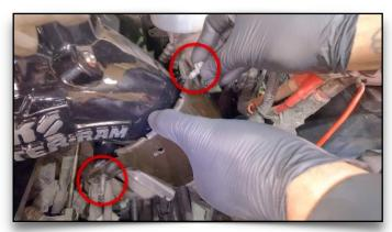
125. Install Throttle Heat Shield Bolt & Nuts
