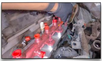
84. Release Bungee Cord. Place Fuel Rail & Studs in Place
