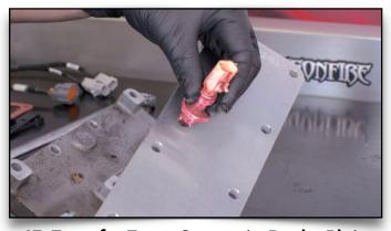
**67. Transfer Temp Sensor to Banks Plate**
