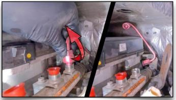
**58. Loosen #6 Fuel Line, Rotate Out of Way** Do not fully remove the rear fuel rail. It is difficult to reach and only needs to be moved out of the way as shown.
