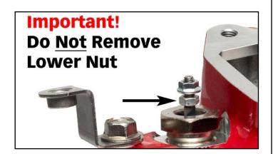
If installing with the Banks High-Flow heater and Billet Plate, the lower locking nut must not be removed from the heater coil. Take care when installing OEM heater wire ring terminal, it must be sandwiched between lower and upper nut.
