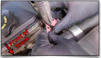
113. Remove & Discard 12V Heater Cable P-Clamp
