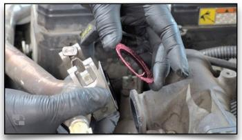
**24. Release Clamp and Remove Gasket** Catch the gasket and put it aside for later, this will be used again.
