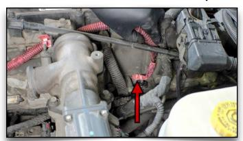
**30. Remove Heater cable from Terminal** Relocate the wire out of the way once the free.
