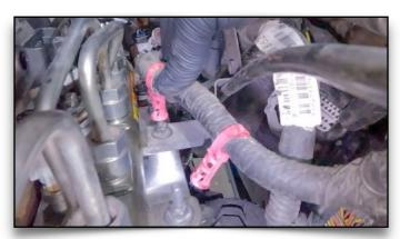
91. Push Engine Harness Cable Ties Back Onto Studs
