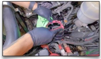
101. Remove Rag From Boost Tube, Put Clamp Back On
