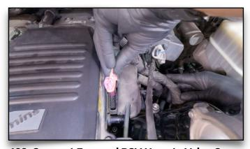
**109. Connect Forward PCV Hose to Valve Cover** This is a tight fit, but doable. Wiggle the rubber hose on
