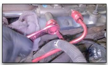
88. Tighten Fuel Supply Line Banjo Bolt Hand Tight. Tighten Fuel Feed Line to 30ft/lb
