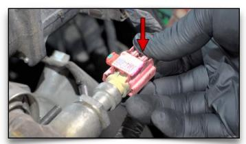
**17. Remove Temp Sensor by Pinching It** Unclip this wire clip for extra clearance.
