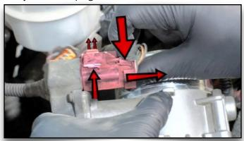
Slide tab over and depress the end to remove the plug.
