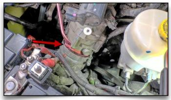
34. Pry Boost Tube Hose Off Throttle Body
