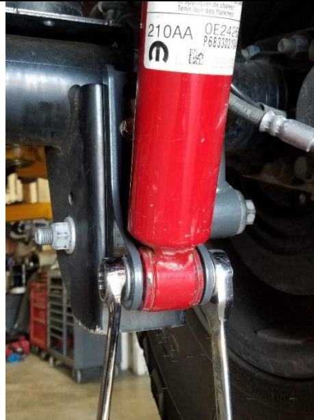
Figure 11. Installing the Shocks
