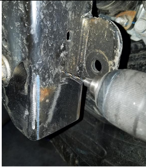
Figure 9. Drilling the Control Arm Bracket
