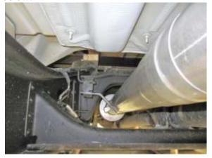
3. Install muffler # 6185, as well as over the axle pipe # 11725, placing metal hanger into OEM isolator.
