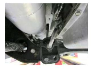
2.Installation of FLO-PRO system. Install pipe # 11711 with 4 hole flange by placing welded metal hanger into OEM transmission isolator as shown above. Loosely snug up 4 fasteners at downpipe (making sure that factory gasket is in place first). Install pipe # 11712 and # 11713, making sure to install hanger on 11713 into OEM isolator as shown below.
