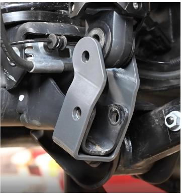
**Figure 2. Shock Extensions Installed**
