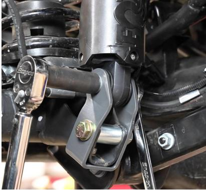
**Figure 3. Bolting Shock to Extension**
