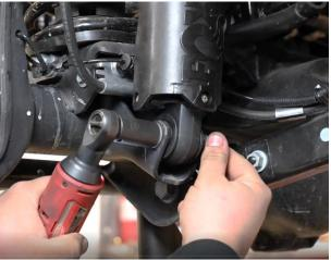
Figure 1. Removing Lower Shock Bolt
