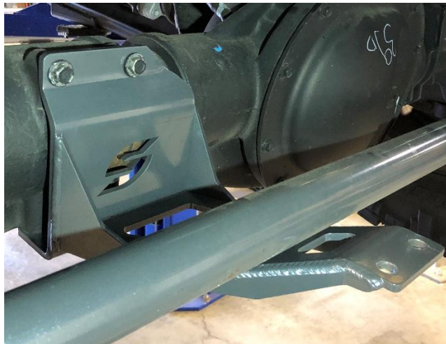
Figure 3. Loosely Installed Synergy MFG Dual Stabilizer Bracket
