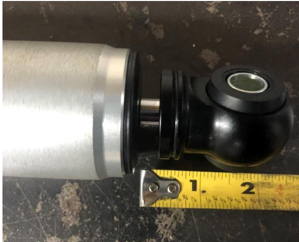
Figure 6. Compressed Steering Stabilizer
