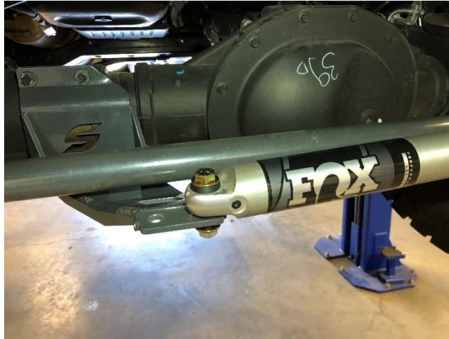
Figure 4. Partially Installed Driver side Stabilizer on Synergy MFG Bracket
