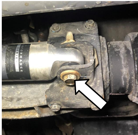
Figure 1. Stabilizer Bolt to be Removed
