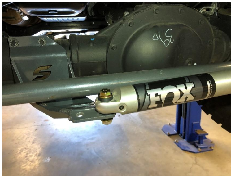
Figure 10. Driver Side Steering Stabilizer Installed on Dual Stabilizer Bracket
