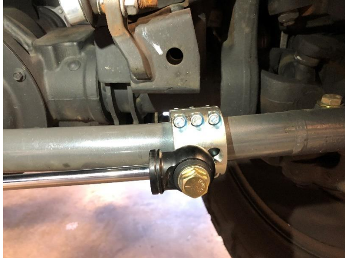
Figure 9. Installed Drivers Side Tie Rod Clamp and Steering Stabilizer
