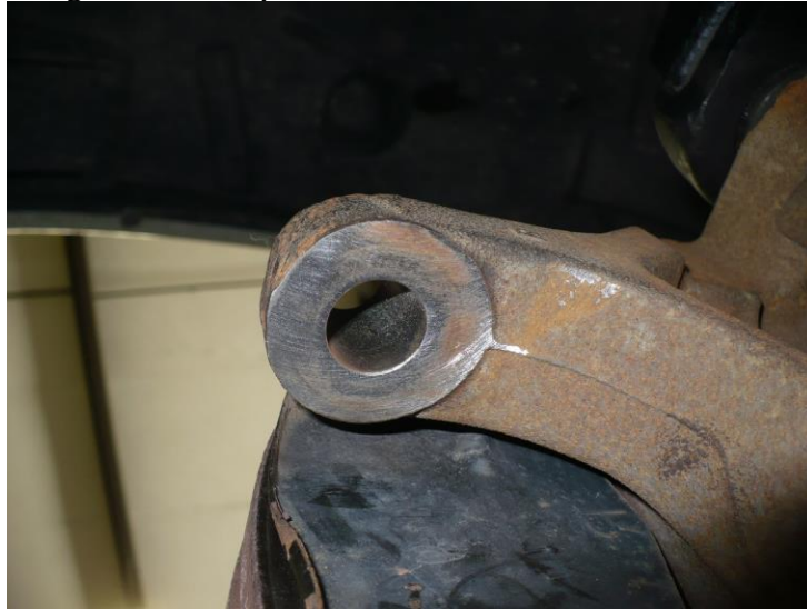
Figure 7. Steering Knuckle Arm Sanded Flat
