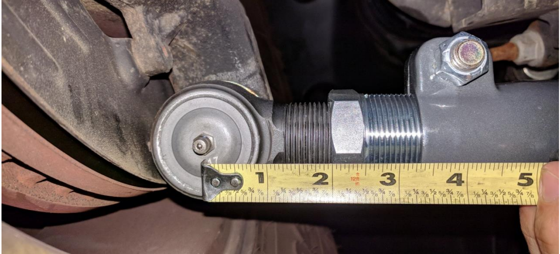
Figure 9. Double Adjuster Tie Rod End Max Extension
