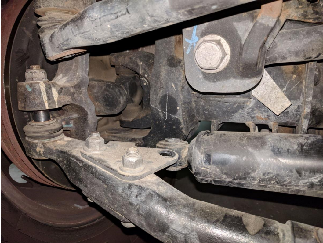
Figure 1. Steering Stabilizer Removed From Stock Tie Rod
