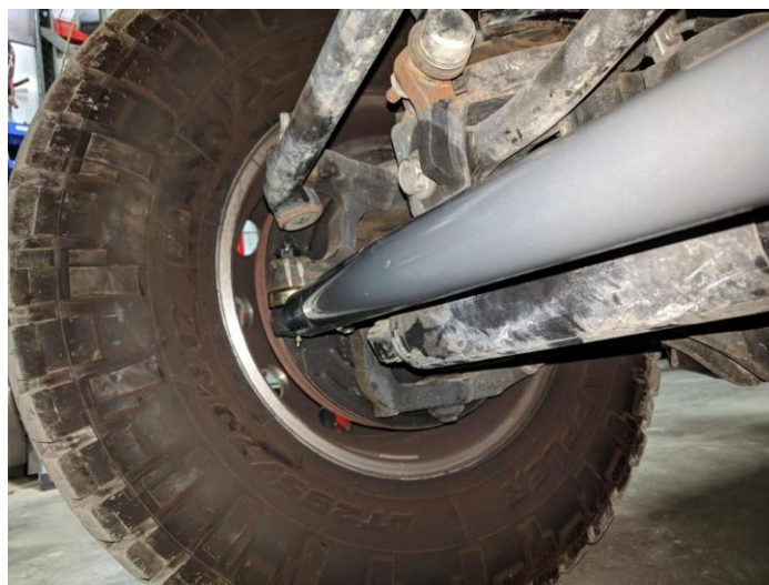
Figure 10. Tie Rod Aligned with Bend Forward and Pinch Bolts Back
