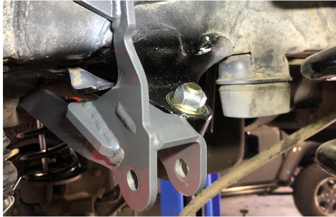
Figure 9. Correctly Installed 5/8" Bolt with Washer on Top Side of Factory Tab
