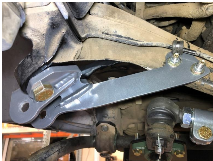
Figure 14. Installed Track Bar Conversion Bracket (Underside View)
