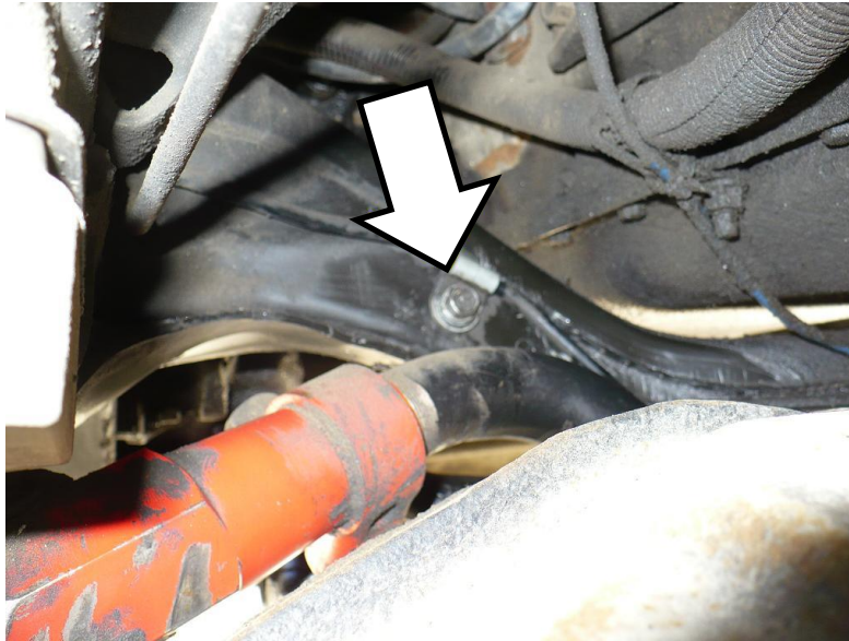
Figure 7. Brake Line Hold Down to be Removed.
