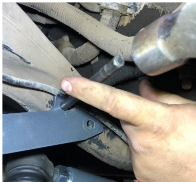
Figures 10 and 11. Center punched and Drilled Crossmember (3/8" Drill Bit)
