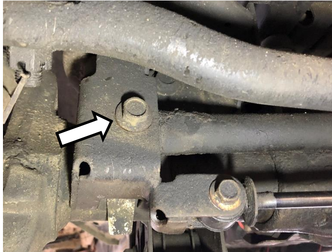
Figure 1. Axle Side Track Bar Bolt
