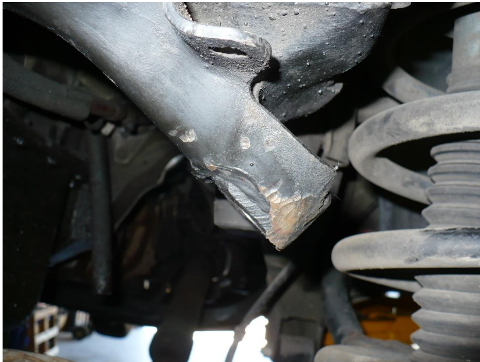
Figure 4. Track Bar Tab that WILL Require Modification
