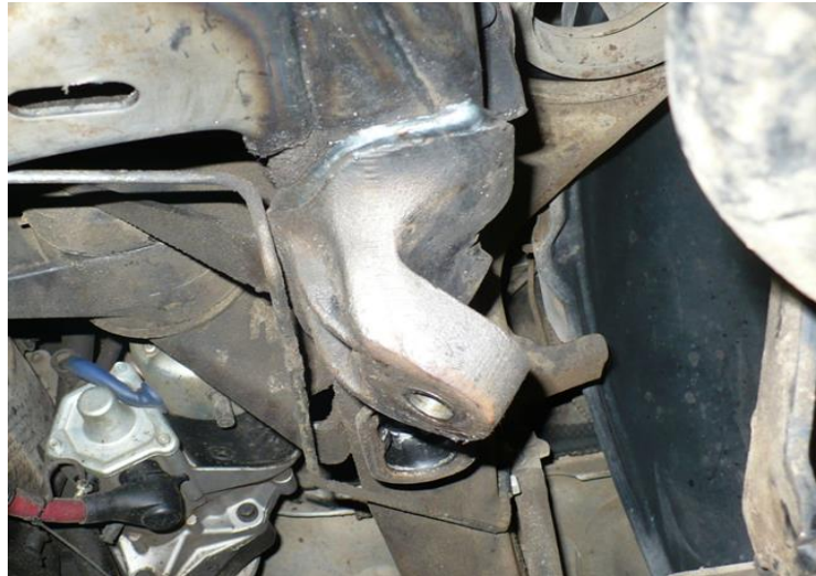
Figure 3. Track Bar Tab that Will Not Require Modification.
