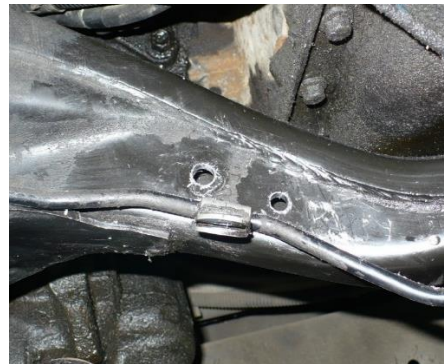
Figures 10 and 11. Center punched and Drilled Crossmember (3/8" Drill Bit)
