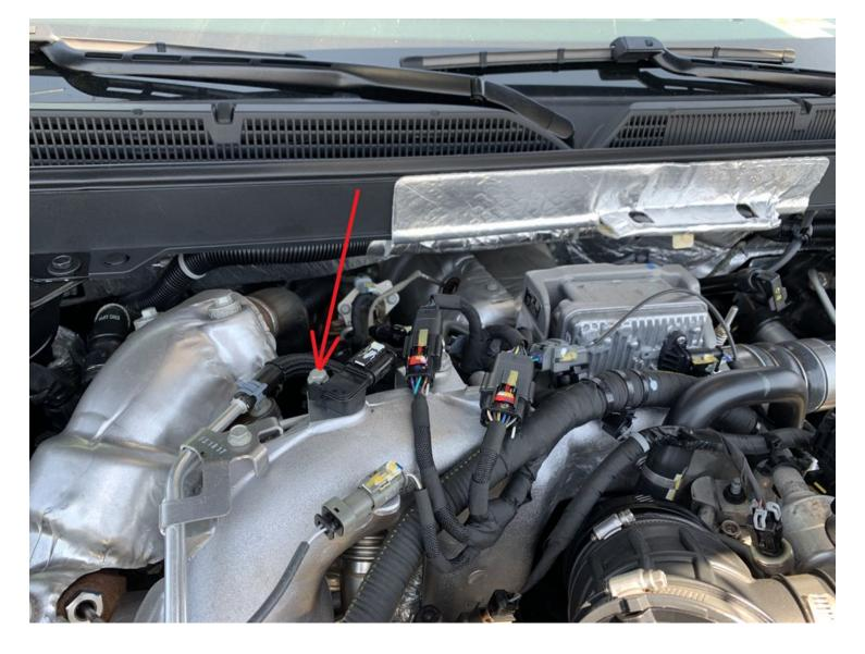
Make sure the engine is off, cooled down, and the vehicle is safely parked with the parking brake set. Locate the MAP Sensor and the M6 Hex Head Flange Screw holding the MAP Sensor in place.
