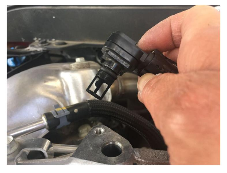
Carefully remove the MAP Sensor from the Intake Manifold. A back and forth twisting helps to make removal easier.
