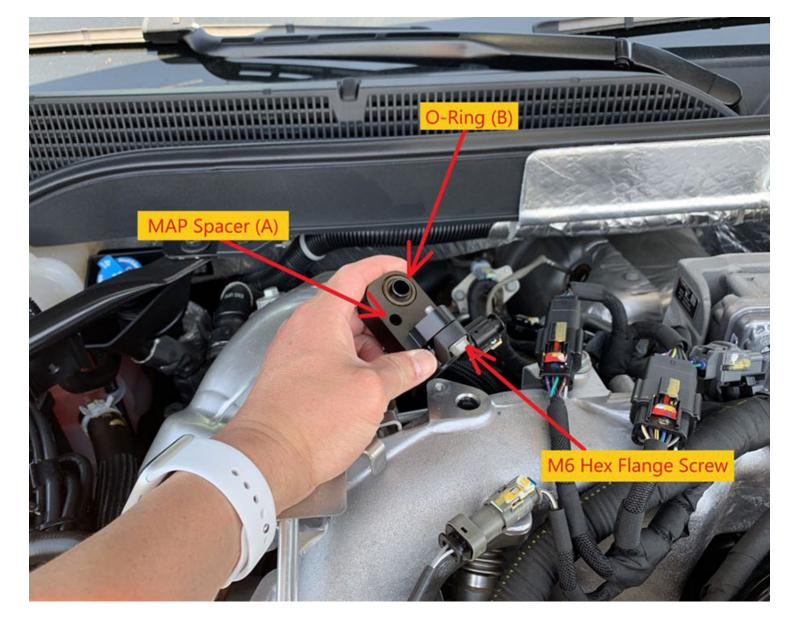
Carefully insert the MAP Sensor into the MAP Spacer (A) and secure it with the M6 Hex Head Flange Screw as shown. Do not use any Threadlocker on this screw and hand tighten only. Install the O-Ring (B) into the Spacer groove. Carefully stretch the O-Ring over the lip to fully seat into the groove. Once fully seated, the O-Ring will stay in the groove as you turn the Spacer over for installation into the Intake Manifold.
