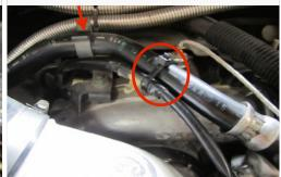
13. Reinstall the S&B intake tube (or the OE intake tube) that was removed in Step #2. Tighten all the hose clamp connections.
