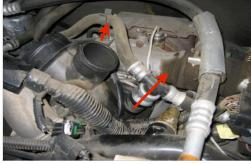
9. Using a needle nose pliers, pull the inner OE hose support out of the CCV hose.
