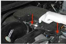
4. Using a 10mm socket, remove the screw mounting the CCV tube on the passenger side. Pull the tube up out of the port. Save the screw for re-mounting.
