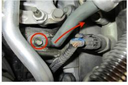
the CCV line from the OE inlet tube.
