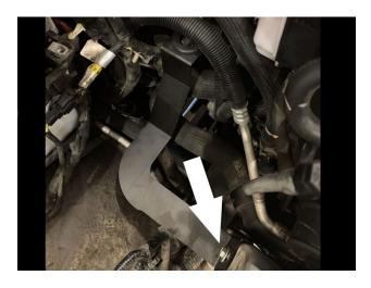
Gently push the AC line so that it sits under the tube support bracket as shown.
