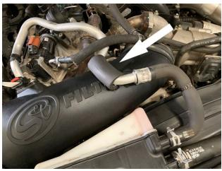
Reconnect the passenger side battery's positive terminal and both battery's negative terminals. Inspect your installation, make sure the kit is properly positioned and all fasteners are secured. S&B Filter recommends keeping all stock parts in case you would ever need to reinstall the stock intake. Affix the ID label near the intake kit. The installation is now complete.
