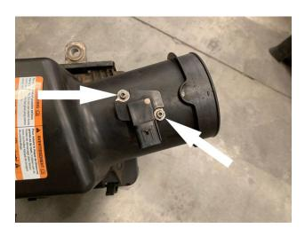
Install the MAF sensor, MAF sensor pad (I) and MAF sensor pad gasket (J) onto the intake tube, securing them to the tube with the provided phillips head screws (H).
