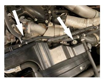
Disconnect all the rubber hoses and coolant lines from the intake tube.
