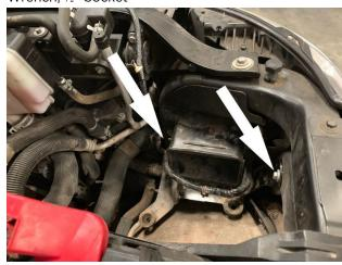
Looking at the top of the engine bay, remove the indicated 4 screws securing the grill to the vehicle.
