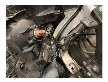
Feed the headlight bulbs through the hole in the engine bay liner so that they are seated inside the engine bay.
