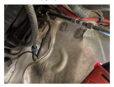
Now that the main heat shield is removed, we can now have access to the fuel lines. Using a small flat head screwdriver or pick, lift on the blue retainer on the connector to unlock and gently pull the fuel lines apart. Repeat this process for the second line. In the same location as the fuel lines, you will notice that there is an electrical plug, this is the connection for the fuel sending unit. Depress the locking tab on the electrical connector and remove.
