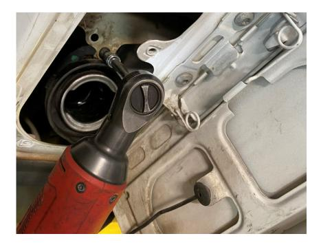
Vehicle is now ready to be lifted in the air and tank removal can begin. Locate galvanized heat shielding on front of the tank, locate the push washers and 10mm mounting bolt. Remove 10mm bolt and use a panel popper tool/flat head screwdriver to remove heat shield retainers. After removal, discard heat shield. It will not be reused.
