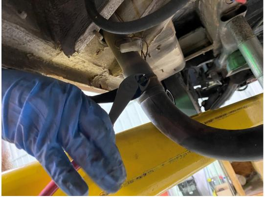
Remove fuel Lines from the top of the tank and disconnect them from the sending unit. The electrical connection will also need to be fully removed. Locate plastic Fuel Hat Torque Ring. Use included removal tool and a 3/8" ratchet to loosen the plastic hold down. Upon removal, discard torque ring and sealing O-Ring.
