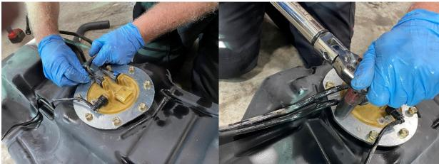
Locate provided filler neck hoses, clamps, and couplers. Assemble the two hoses together with coupler and hose clamps. Identify the hose with a 45-degree angle bend and install metal filler neck inlet and tighten hose clamp. Please note orientation of the mounting hole on top should be at 12 o'clock position. Install supplied vent line hose to metal fill neck vent and tighten provided hose clamp. Install the filler neck assembly on the tank King Nipple and tighten the provided hose clamp.
