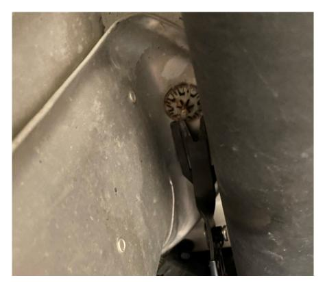
Located under the filler neck is an additional shield with 4 10mm nuts holding it in place.
