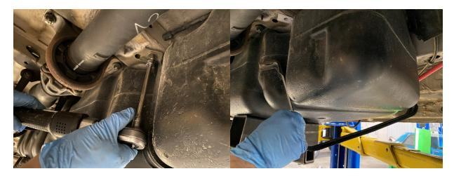
Begin lowering tank slowly, paying special attention so that the filler neck does not hang-up on anything. The filler neck ground connection will need to be unclipped. This is done by pressing the tab down and pulling the two ends apart. The zip tie holding the wire will also need to be cut off. Remove tank from under vehicle and place it next to your NEW XXL TITAN TANK.
