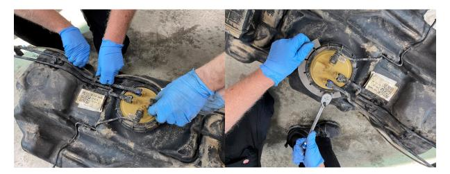
Take new supplied O-Ring and lubricate lightly with clean grease or oil and install into O-Ring gland on top of tank. Transfer sending unit into the Titan Tank. Be sure that the sending unit is clocked in the same location as the factory tank. Install top crash flange and the provided locking nuts. Torque all 8 nuts to 25 LB-Ft of torque in a star pattern. Wait 15 minutes to retorque 25 LB-ft MAX.
