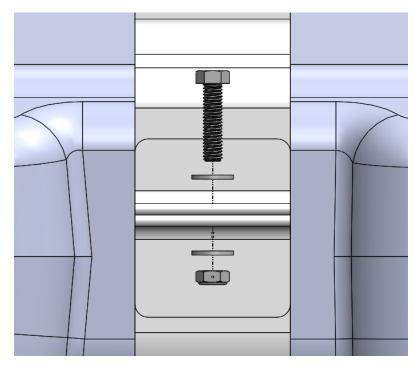
Exploded view of hardware to mount two straps.
