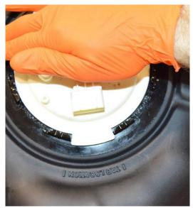
Sample image of sending unit aligned with marking on tank.
