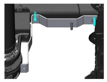
Installed E Bracket for Front Support. If using a plusnut for installation, the bolt on the right will extend up into the crossmember instead of pointing down.
