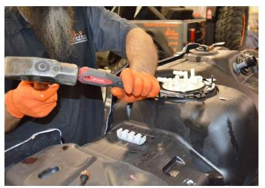
Sample image of removing an OEM lock ring
