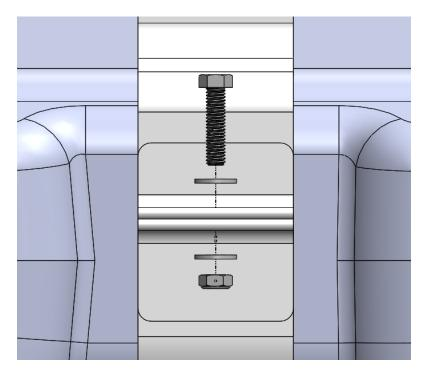
Exploded view of hardware to mount the A (or C) Tab Strap to the B Strap.
