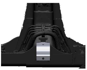
Sample images of an installed C Tab Strap. Actual vehicle may look slightly different.
