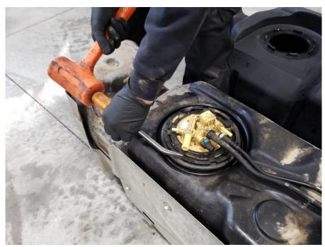
Sample image of removing an OEM lock ring
