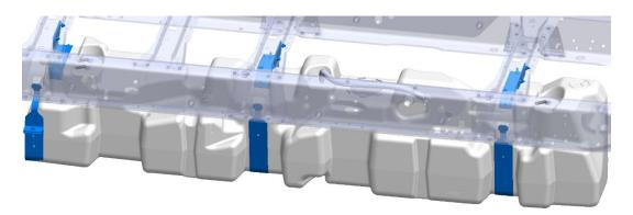
A1 Bracket - Used with Rear Strap on all configurations. 2qty 5/16" Washers and 2qty 5/16"-18 Locknuts will be used. (99 0000 0991 & 99 0000 0455)
