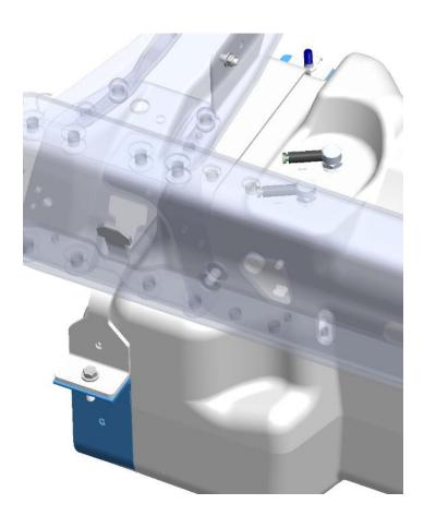
Fully installed G3 Bracket on 120 CA. 1qty 3/8-16 x 1.5" Cap Screw, 1qty U Nut, 3/8"-16 0.75" center and 1qty 3/8"-16 Washer will be used to connect to G1. (02 0000 0456, 02 0000 0428 & 99 0000 0682)
