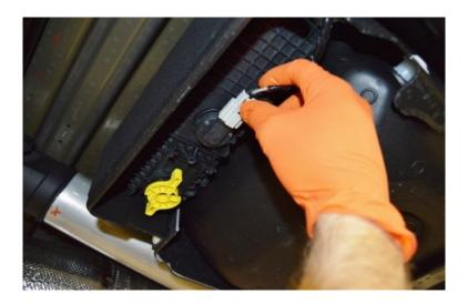
Next, disconnect the fuel line at the top of the separator by squeezing the two legs of the tab together and then pushing the entire tab towards the rear of the vehicle. Note: This coupling operates differently from all others involved in the install.
