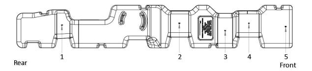
The top brackets and hangers must be installed before the tank body is lifted into the vehicle. These include A1, C, D, G1, and G2. Please view the images below as they depict placement and direction. As stated above, straps and supports will vary depending on application.
