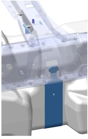
Fully installed A2 Rear Strap on all configurations. 1qty 3/8-16 x 1.5" Cap Screw, 1qty U Nut, 3/8"-16 0.75" center and 1qty 3/8"-16 Washer will be used. (02 0000 0456, 02 0000 0428 & 99 0000 0682)
