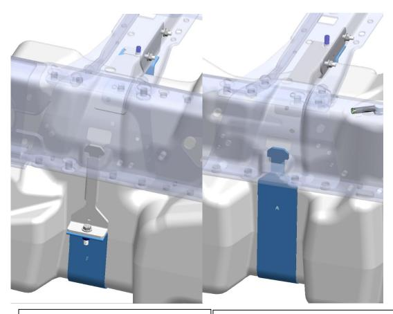
Fully installed F Front Strap. 1qty 3/8-16 x 1.5" Cap Screw and 1qty 3/8"-16 Washer will be used. (02 0000 0456 & 99 0000 0682)
