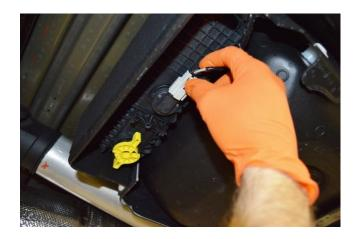
9 Next, disconnect the fuel line at the top of the separator by squeezing the two legs of the tab together and then pushing the entire tab towards the rear of the vehicle. Note: This coupling operates differently from all others involved in the install.
