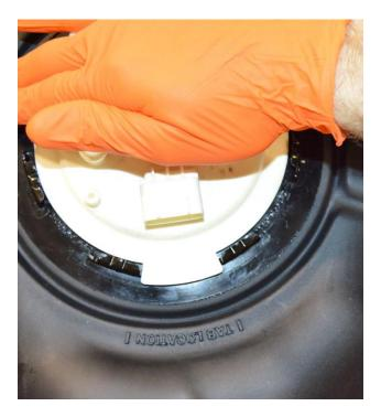
19 Place the hold down ring from the OEM tank onto the sending unit and tighten it clockwise as far as it will go.
