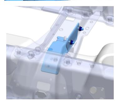
Fully installed D Tab for the front strap. (Used on all configurations)
