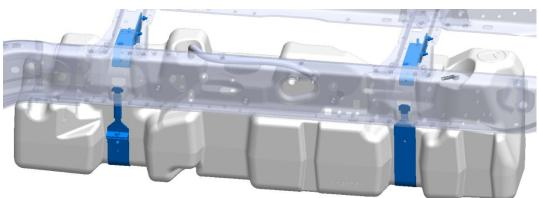
Fully installed A1 Bracket for the rear strap. 2qty 5/16" Washers and 2qty 5/16"-18 Locknuts will be used. (99 0000 0991 & 99 0000 0455)
