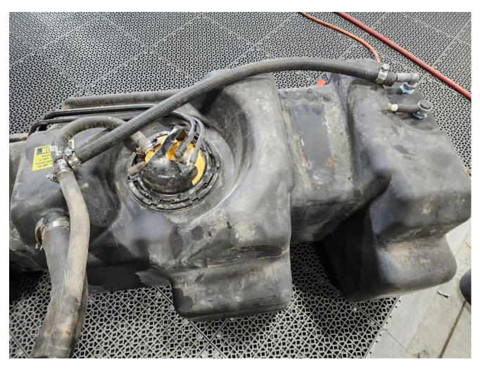
Insert 1-1/2" Fill Pipe ICV into the tank side of the fill hose. The "Flow" arrow will need to be pointing towards the fuel tank. This will need to be inserted deep enough to allow the fill hose to fit completely over the king nipple.
