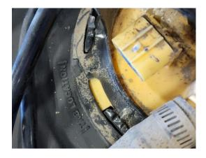
Lay the fuel lines into the fuel line groove provided in the top of the replacement tank.
