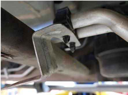
Install tank front support according to the images below. The short bed configuration will have the front support pointing towards the front of the truck. The standard bed configuration will have it pointing towards the rear.
