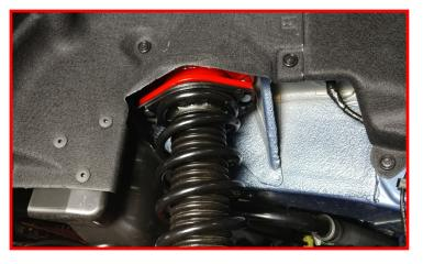
Raise the lower control arm into place and install the lower strut hardware. Do not tighten at this time. Use the jack and raise the lower control up to set pre load on the strut. Install the lower knuckle bolt. Do not tighten at this time.
