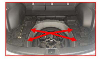
Remove the strut covers by pulling upwards at the trunk area, then pushing down at the plastic cover, and set aside.
