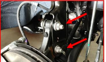
Locate the ReadyLIFT front strut extension. These are driver and passenger side specific and have a D and P etched into the top. Passenger side shown. Install to the top of the strut using the factory hardware. Torque to 30 ft-lbs.
