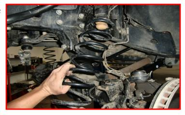
Locate the ReadyLIFT front bump stops onto the center of the axle pad. Use a punch to mark the pad for drilling.
