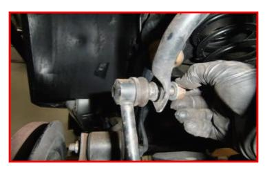
Lower the axle enough to remove the springs from the vehicle. Be careful to not overextend the brake lines and ABS harness.
