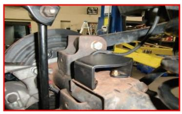
Install the ReadyLIFT rear springs using the factory isolator. Raise the axle up enough to hold the springs in place. Install the provided shocks with the factory hardware. Torque the upper to 35 ft-lbs. Do not tighten the lower at this time.
