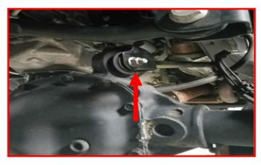
Loosen but do not remove the lower control arm bolts at the axle.
