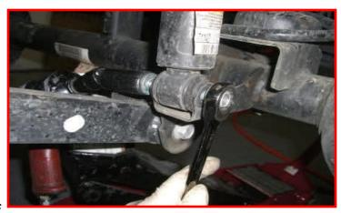
Remove the front sway bar end links from the axle and sway bar. Mark the front driveshaft to pinion location. Remove the front driveshaft hardware. Let hang out of the way.
