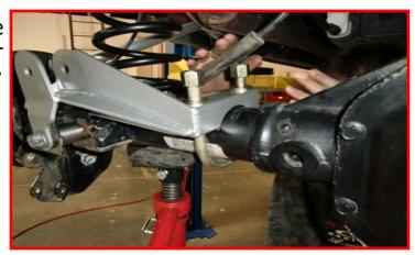
Install the track bar to the bracket using the provided hardware. Do not tighten at this time.
