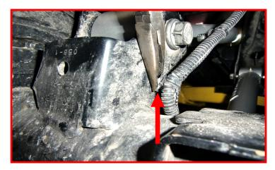
Locate the E-brake cables above the axle and remove the bracket from the body tub. Let hang out of the way.
