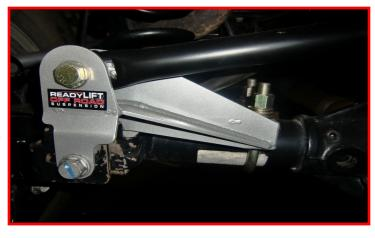
Install the ReadyLIFT rear bump stops using the provided hardware. Torque to 15 ft-lbs.
