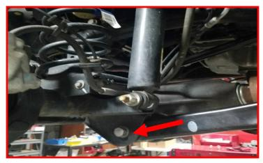
Locate the upper control arms where they meet the frame. Remove the bolt that holds the heat shield to the frame.
