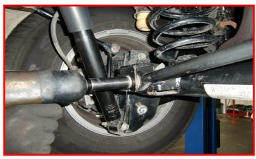
Remove the sway bar end links from the axle and the sway bar.
