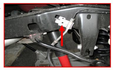
Remove the ABS harness clips from the axle and frame rail. Let hang out of the way.
