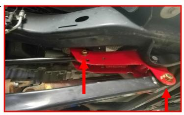
Support the axle with a suitable jack. Remove the front brake line brackets at the axle and frame rail. Let hang out of the way. Remove the vent tube from the driver side spring mount. Let hang out of the way.
