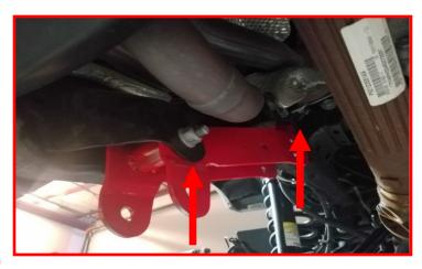
Install the upper arm to the bracket (use the upper hole for 2.5" lift heights, and lower hole for 3-4" lift heights) using the provided M12 x 80 mm bolts, washers, and nuts. Install the lower control arm to the bracket using the provided M14 x 100 mm bolts, washers and nuts. Do not tighten at this time.
