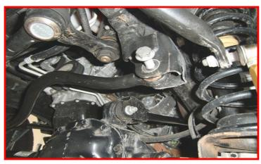
Lower the axle low enough to remove the front springs.
