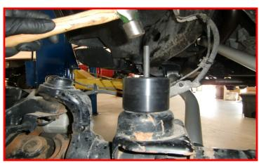
Use a suitable drill, drill out the previously made mark using a 3/8" drill bit.
