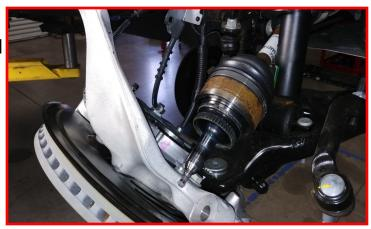
Support the lower control arm with a suitable jack. Loosen but do not remove the lower control arm to frame mounting hardware. Remove the lower strut from the lower control arm. Remove the sway bar end link from the lower control arm.
