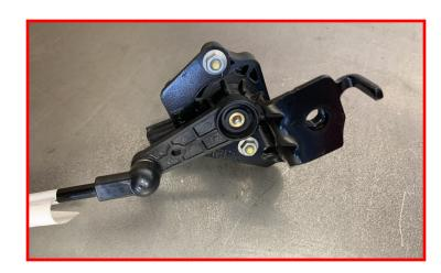
Install the replacement CCD control potentiometer mounting bracket in the factory orientation using the factory hardware.
