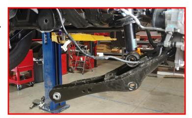
Locate the ReadyLIFT strut spacer. Install using the provided M10 - 1.5 flange nuts.
