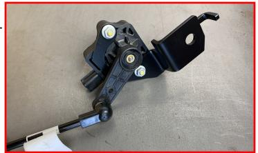
Install the replacement CCD control potentiometer mounting bracket into the frame in the factory orientation. Install using the factory bolt and the supplied M8 locking nut and flat washer.
