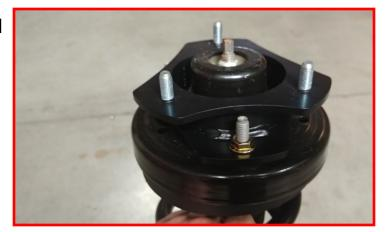
Install the completed strut assembly into the frame using the provided M10 - 1.25 flange nuts. Do not tighten at this time.
