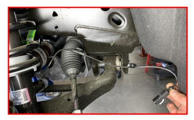
Support the lower control arm with a suitable jack. Loosen but do not remove the lower control arm to frame mounting hardware. Remove the (2) lower strut mounting nuts from the lower control arm. Remove the (3) top strut mounting nuts. Remove the sway bar end link from the lower control arm.
