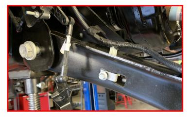
Connect the CCD solenoid harness connector located on the side of the frame behind the strut towers.
