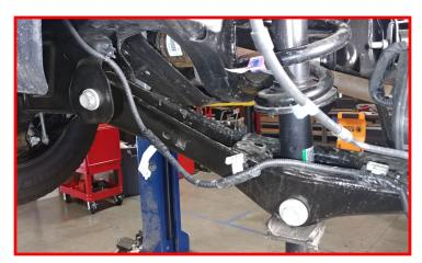
Tighten the (3) M10 - 1.25 flange nuts on the top of the rear strut spacer.
