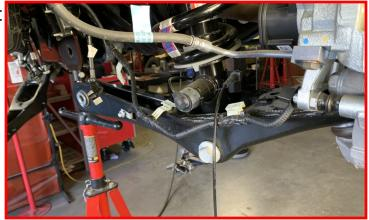
Carefully jack the lower control arm back into the frame.
