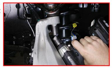
Loosen but do not remove the upper control arm pivot hardware. Raise the upper control arm up and tilt the knuckle away from the frame. Carefully disengage the CV axle from the hub and actuator. Be careful not to damage the Vacuum actuator. The internals are made of plastic and easily damaged.
