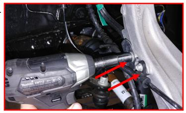
Install the brake line bracket to the frame rail using the factory hardware. Torque to 5 ft-lbs. Install the ABS harness to the frame rail, brake line bracket, and rubber brake line using the factory clips.
