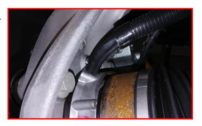
Install the brake line bracket and ABS harness to the knuckle using the factory hardware.
