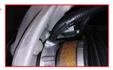
Install the brake line bracket and ABS harness to the knuckle using the factory hardware. Torque all to 5 ft-lbs.
