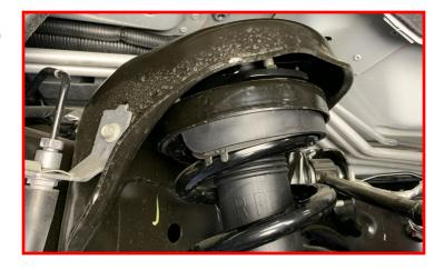
Install the lower strut hardware but do not tighten at this time.
