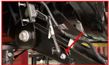
Disconnect the CCD solenoid harness connector located on the side of the frame behind the strut towers.
