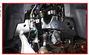
Install the ReadyLIFT front strut spacer using the factory hardware. Torque to 30 ft-lbs.
