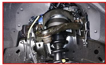
Raise the lower control arm up while guiding the lower strut into place. Install using the factory hardware. Install the sway bar end link using the factory hardware. Torque all to 45 ft-lbs.
