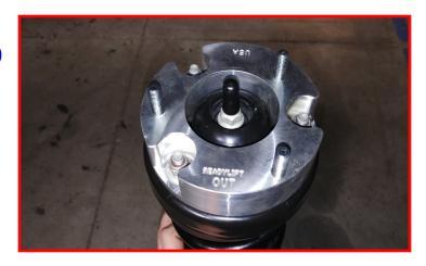
Place the completed strut assembly cross pin studs loosely into a vice or other suitable device. Note the angle the strut is leaning. Push on the top of the strut until the same angle is achieved the opposite direction. This is setting the cross pin studs into the proper orientation for installation.
