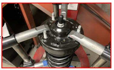
Install the ReadyLIFT front strut spacer using the factory hardware. Torque to 30 ft-lbs.
