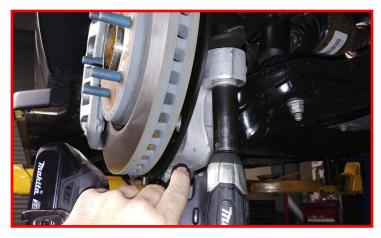
Remove upper ball joint from the knuckle. Strike the ball joint boss with a dead blow hammer to dislodge the taper.
