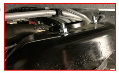
Install the control potentiometer bracket on the rear lower control arms.
