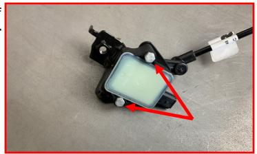
Remove the CCD control potentiometer mounting bolts. Retain the factory hardware.
