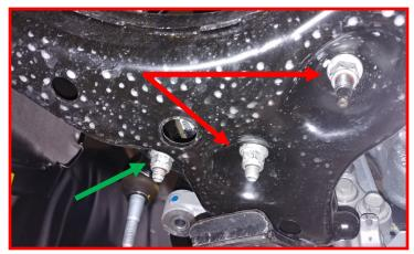
Carefully lower the control arm and knuckle assembly down until the strut clears the control arm. Make sure to not over extend the brake lines and ABS harness. Adjust as necessary. To aid in removal, push knuckle towards the frame as you lower the control arm. Remove the strut from the vehicle by undoing the upper strut hardware.
